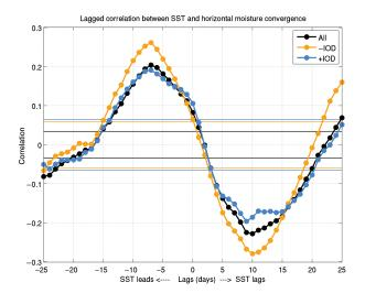
**Figure 6.** Lagged correlations between SST and horizontal moisture convergence averaged over the northern BoB (85°-95°E, 15°-25°N), color-coded to represent the correlations during all, -IOD and +IOD years. The horizontal lines represent the lower and upper 95% confidence bounds for each case
