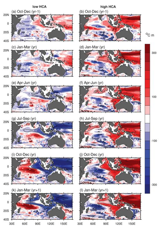
FIG. 9. Evolution of Indian Ocean heat content anomalies in the control simulations: composite anomalies of seasonal heat content ( $^{\circ}C$  m) leading into (yr-1) and out of (yr+1) (left) low and (right) high heat content events (yr), as defined in the control simulation for the period 1970–2004. The area enclosed by the dashed contours denotes anomalies that are significant at the 90% level as estimated by a two-tailed *t* test.
