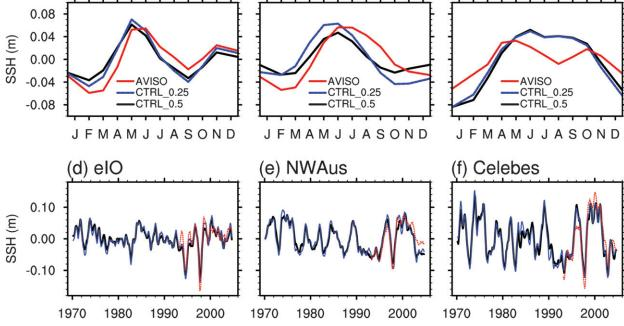
FIG. 10. Observed and model variability in SSH in key regions around the Maritime Continent: (a)–(c) seasonal cycle of SSH and (d)–(f) SSH time series for the three different regions indicated in Fig. 3. SSH is based on control model simulations at  $0.5^{\circ}$  (black) and  $0.25^{\circ}$  (blue) horizontal resolution, as well as observed SSH from AVISO (red). With the exception of the observations (1993–2004), the analysis period covers 1970–2004.
