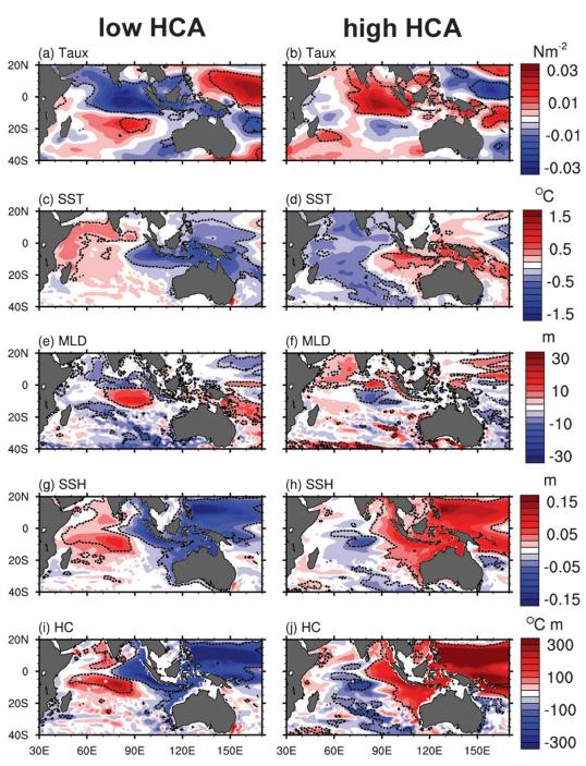
FIG. 6. Composite anomalies in the control simulation for the period 1970–2004 for (left) anomalous low and (right) anomalous high eIO heat content events. Anomalies are shown for (a),(b) zonal wind stress (N m<sup>-2</sup>); (c),(d) SST (°C); (e),(f) mixed layer depth (m); (g),(h) SSH (m); and (i),(j) heat content (°C m). The area enclosed by the dashed contours denotes anomalies that are significant at the 90% level as estimated by a two-tailed *t* test.
