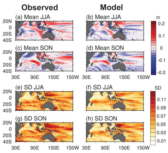
FIG. 3. Comparison of model and observed SSH in the Indo-Pacific: (a)–(d) seasonal deviation from the long-term mean and (e)–(h) seasonal standard deviation, for (left) observed and (right) control simulation for the period 1993–2004. The boxes in (h) indicate regions used for further time series analysis: namely, eIO (box I), NWAus (box II), and Celebes (box III).
